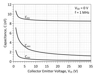
Figure 16: Typical C-V Characteristics
