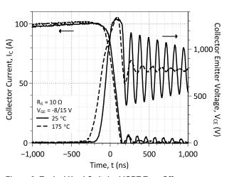
Figure 8: Typical Hard-Switched IGBT Turn Off Waveforms
