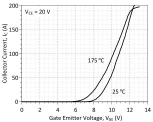
Figure 3: Typical Transfer Characteristics
