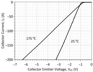
Figure 5: Typical FWD Forward Characteristics
