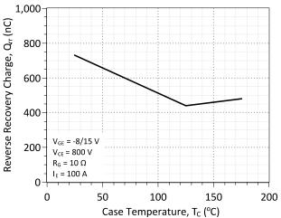
Figure 15: Typical Hard-Switched Reverse Recovery Charge vs. Temperature
