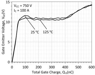
Figure 6: Typical Turn On Gate Charge
