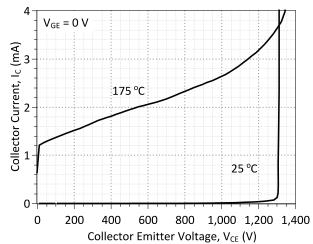
Figure 4: Typical Blocking Characteristics
