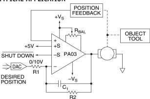
The PA03 output power stages contain fast reverse recovery diodes for sustained high energy flyback protection.
