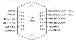
Pins 6 & 7 must be connected together.
