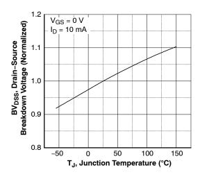
Figure 7. Breakdown Voltage Variation vs. Temperature
