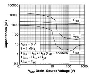
Figure 5. Capacitance Characteristics
