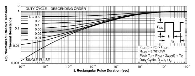
Figure 12. Transient Thermal Response Curve
