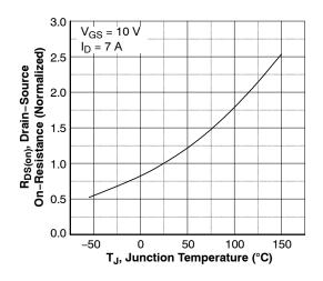
Figure 8. On–Resistance Variation vs. Temperature
