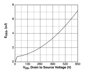
Figure 11.  $E_{\mbox{OSS}}$  vs. Drain to Source Voltage
