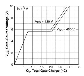
Figure 6. Gate Charge Characteristics
