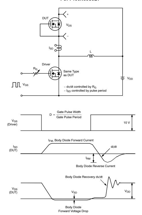
Figure 16. Peak Diode Recovery dv/dt Test Circuit & Waveforms
