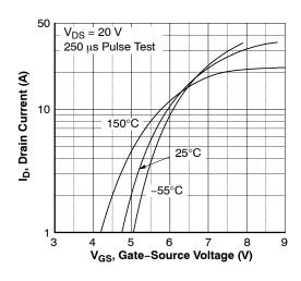
Figure 2. Transfer Characteristics
