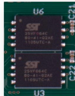
The serial FLASH devices are connected to the **RSPI0** port of the RX MCU:
