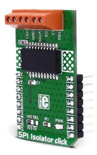
**SPI Isolator click** carries the ADuM4154 **5kV** digital isolator optimized for a serial peripheral interface (SPI). The click is designed to run on either 3.3V or 5V power supply. It communicates with the target microcontroller over SPI interface.
