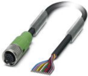
Sensor/actuator cable, 12-position, PUR halogen-free, black RAL 9005, free cable end, on Socket straight M12 SPEEDCON, A-coded, cable length: 5 m
