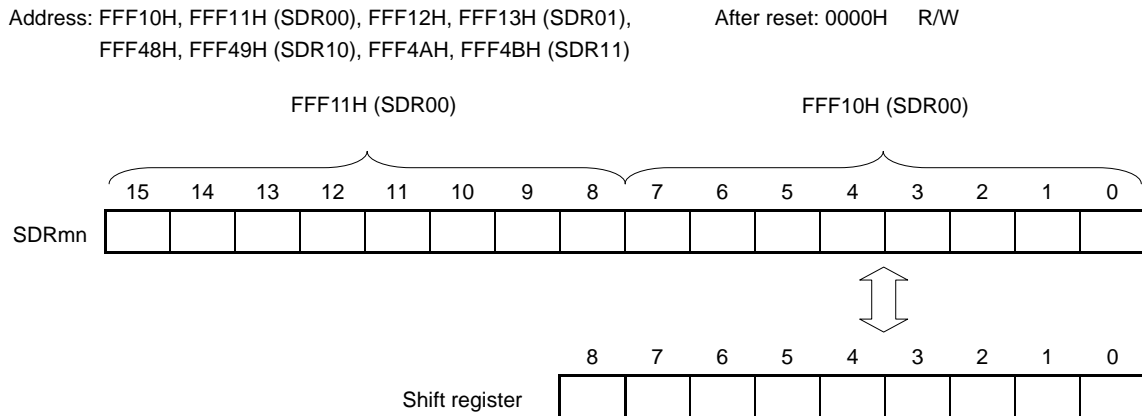
Figure 14-3. Format of Serial Data Register mn (SDRmn) (mn = 00, 01, 10, 11)
