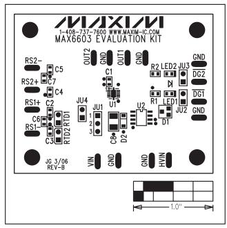
Figure 2. MAX6603 EV Kit Component Placement Guide—Component Side
