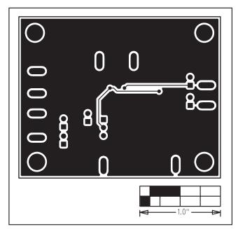
Figure 4. MAX6603 EV Kit PC Board Layout—Solder Side
