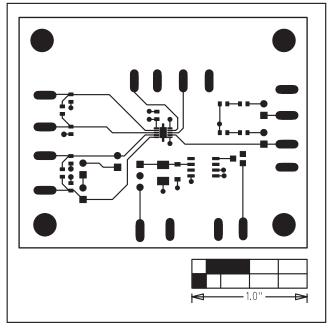
Figure 3. MAX6603 EV Kit PC Board Layout—Component Side
