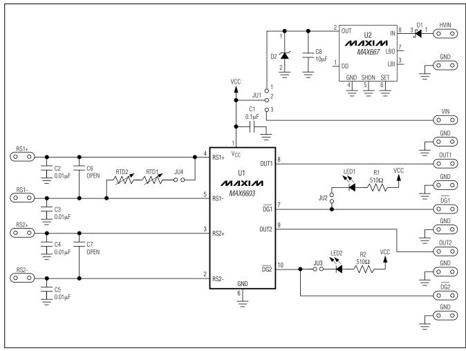
Figure 1. MAX6603 EV Kit Schematic
